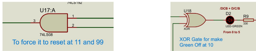
Figure 2: Added detail images. Left: 74LS08 gate used to force reset at 11 and 99. Right: XOR gate used to force the green LED OFF at 10.
