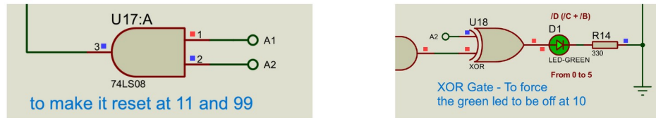
Figure 2: Additional notes supplied for this update. Left: U17:A 74LS08 reset gate to force reset at 11 and 99. Right: U18 XOR gate to make the green LED OFF at 10.
